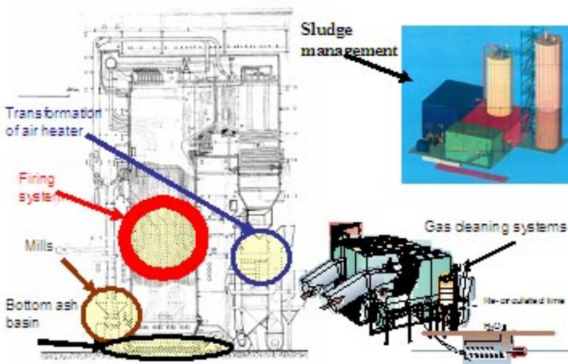
Figure 18: Transformation areas of No 3 power plant unit in Aliveri
