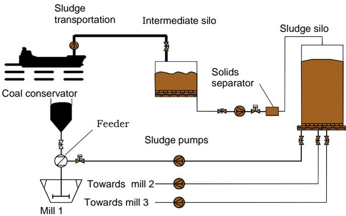
Figure 17: Flow chart of sludge management in the power plant of PPC in Aliveri
