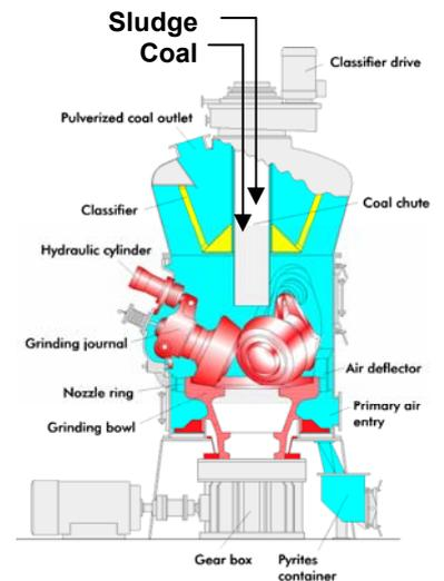
Figure 19: Co-firing of sludge & hard-coal in hard-coal fired power station
