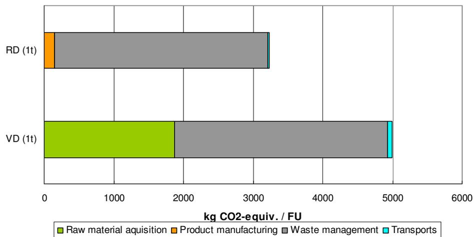
Figures 2a – 2c CO<sub>2</sub>-equivalents from the product systems studied. Abbreviations: PLPC = Plastic profile combustion, PLPL = plastic profile landfill, IW = impregnated wood, RT = recycled textile mat, PP = polypropylene mat, RD = recycled plastic drainpipe, VD = virgin plastic drainpipe, FU = functional unit (100m<sup>2</sup> or 1t). Note that the pillars do not include any emissions avoided by energy recovery of waste.
