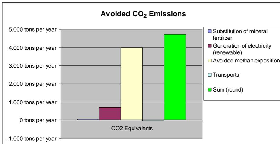
Fig. 4 Avoided CO<sub>2</sub>-Emissions of the Demonstration Plant
