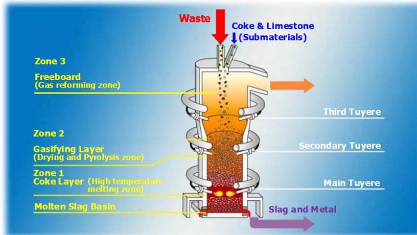
Fig. 2 - Structural drawing of Gasifying and melting furnace
