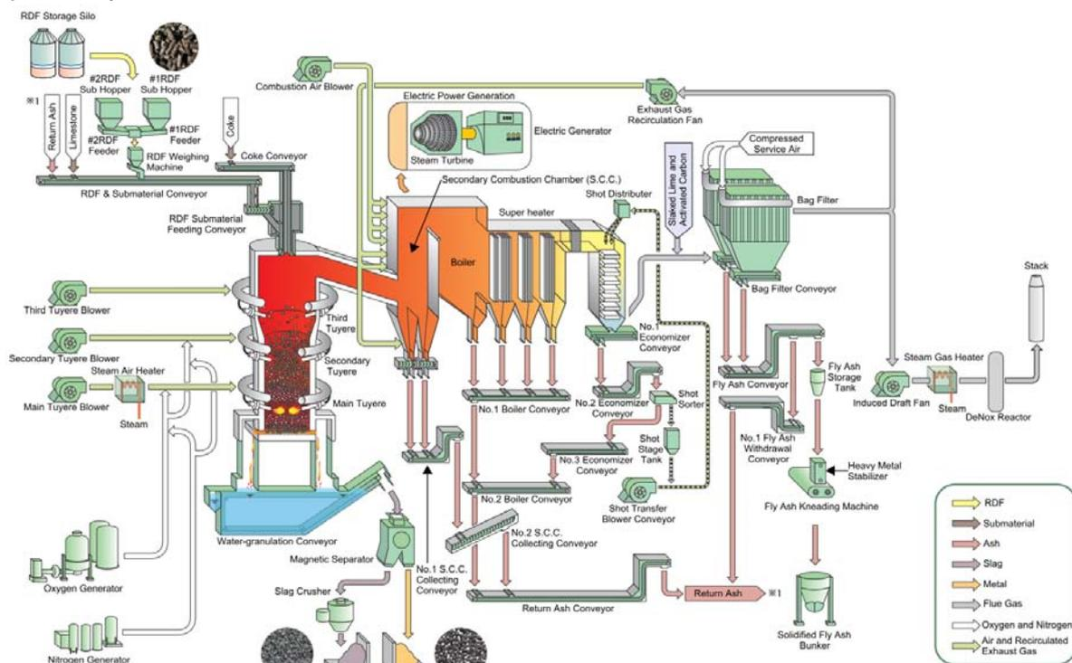
Fig. 3 - Process Flow of Fukuyama Recycle Power
